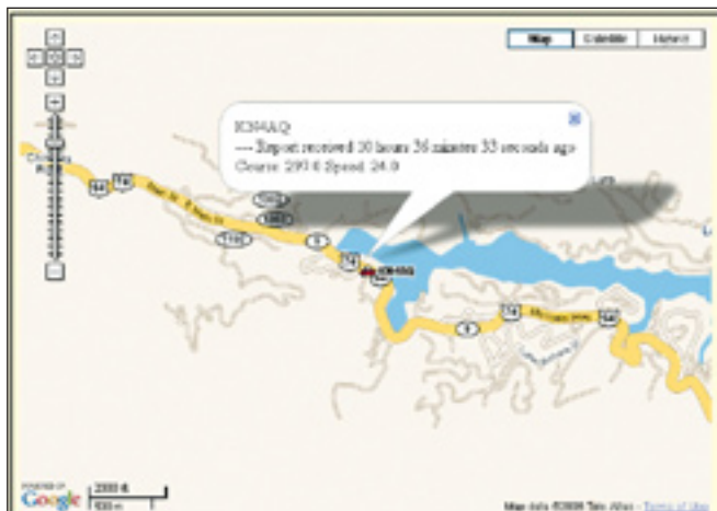
Figure 6 — My position, course and speed, as reported on FindU.com, courtesy of the Dplus program running on the Charlotte D-STAR Gateway.
